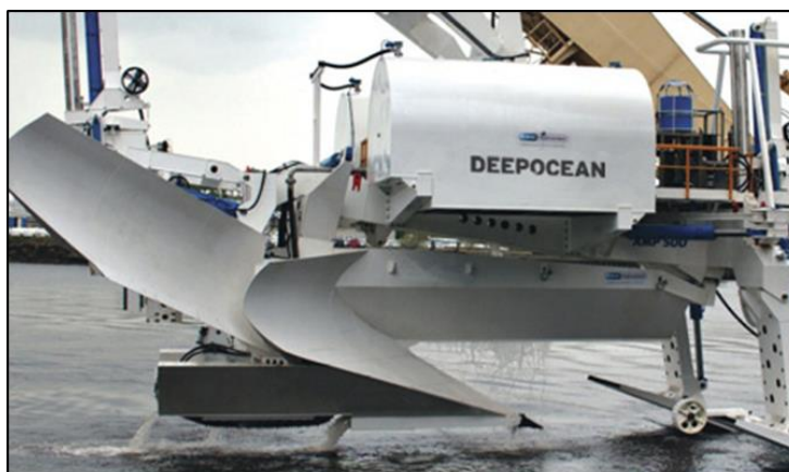
Figure 13: Deep Ocean AMP500 Plough
